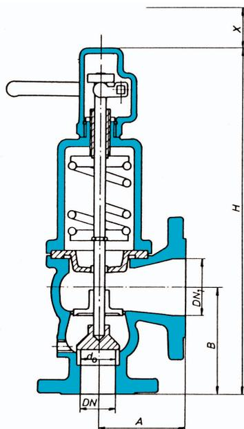
with closed protective bonnet and closed lift housing
