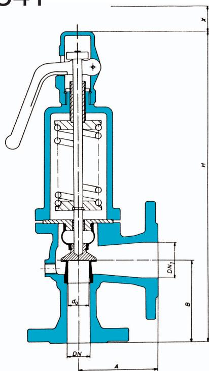
with closed protective bonnet and open spindle housing cap
