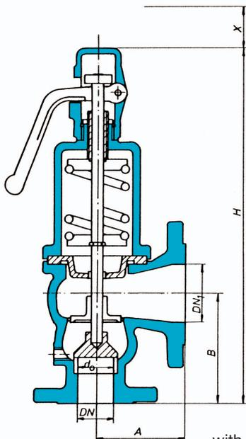
with closed protective bonnet and open lift housing
