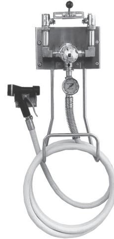
Unit is supplied fully assembled and pressure tested with strain relief and 20 mm coupling for hose attachment. Inlet check valves are required (not supplied).
