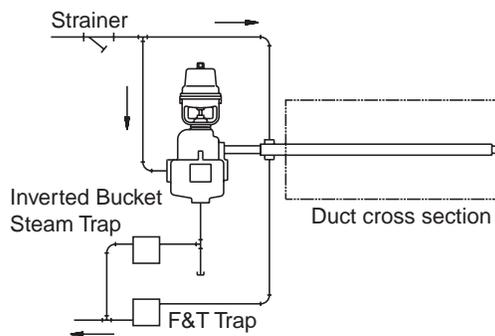
**Figure 59-3. Steam supply direct to separator (Manifold trapped separately)**
