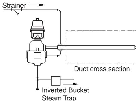
**Figure 59-2. Steam supply direct to separator (Manifold trapped separately)**
