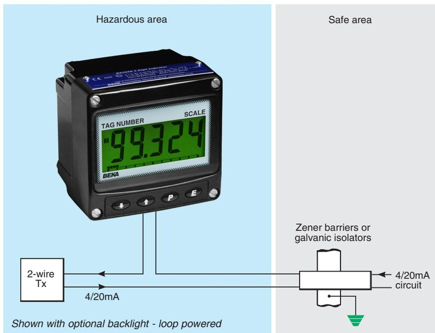
The **BA324G loop powered 4/20mA indicator** is a new field mounting instrument that supersedes the well established BA324C. It is electrically and mechanically compatible with the earlier model but has a much larger full 5 digit display and guaranteed performance between  $-40$  and  $+70^{\circ}\text{C}$ . Like its predecessor, the BA324G is housed in a robust IP66 enclosure which may be surface or pipe mounting.
