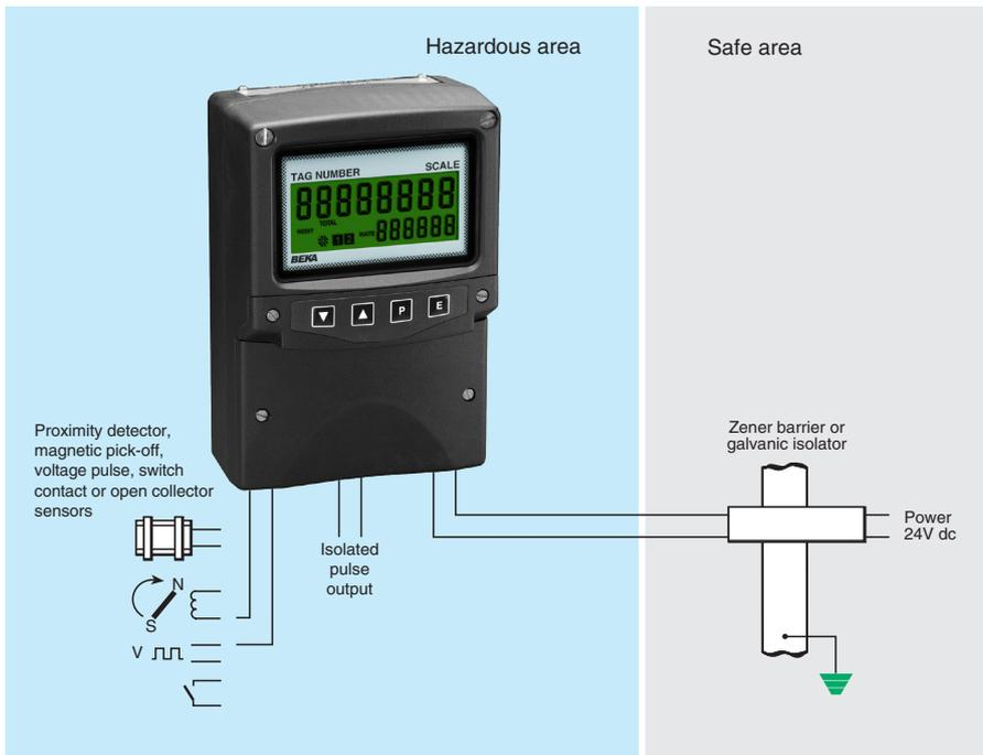
The **BA334E** is a third generation intrinsically safe field mounting rate totaliser housed in a robust IP66 GRP enclosure with a separate terminal compartment. The totaliser is easy to use and can be configured on-site to operate with flowmeters having a magnetic pick-off, switch contact, proximity detector, open collector or a voltage pulse output. International intrinsic safety certification permits worldwide installation.
