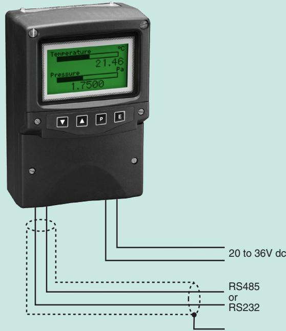
The **BA684D** is a dc powered instrument that can display text and simple graphics in a process area. Incorporating four push-buttons and two single pole outputs, the BA684D is a low cost robust operator interface ideal for simple machine and process control applications.
