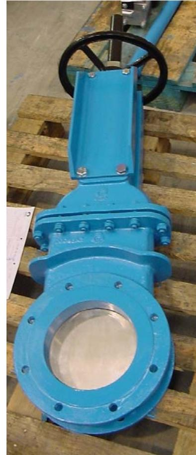
**Note:** These pressures are to be applied on the valve following the direction of the arrow stamped on the body side. Due to the valve design with seating wedges it is allowed 50% of these pressures in the opposite direction of the arrow. Bidirectional design also available under request
