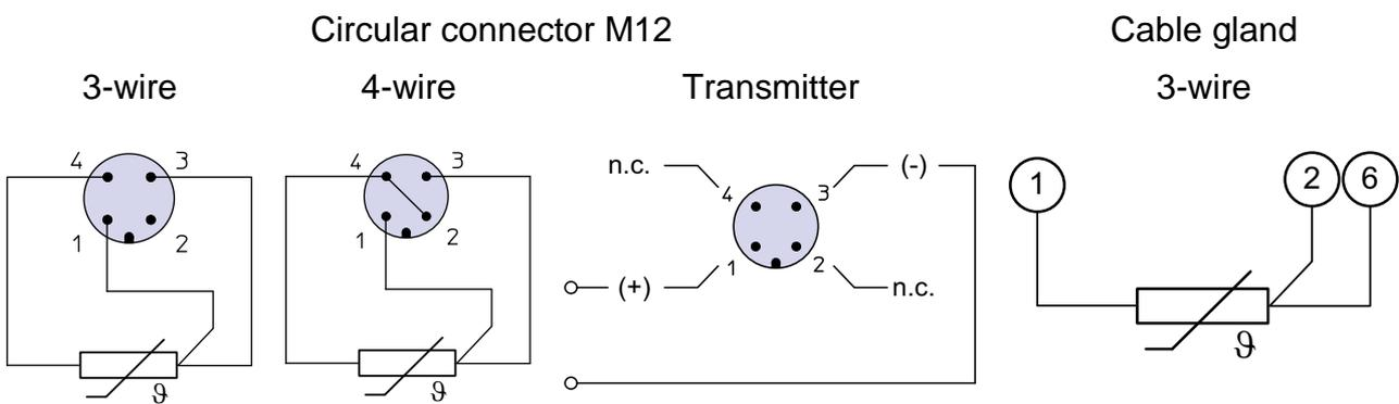
Figure 1: Variants of electrical connection
