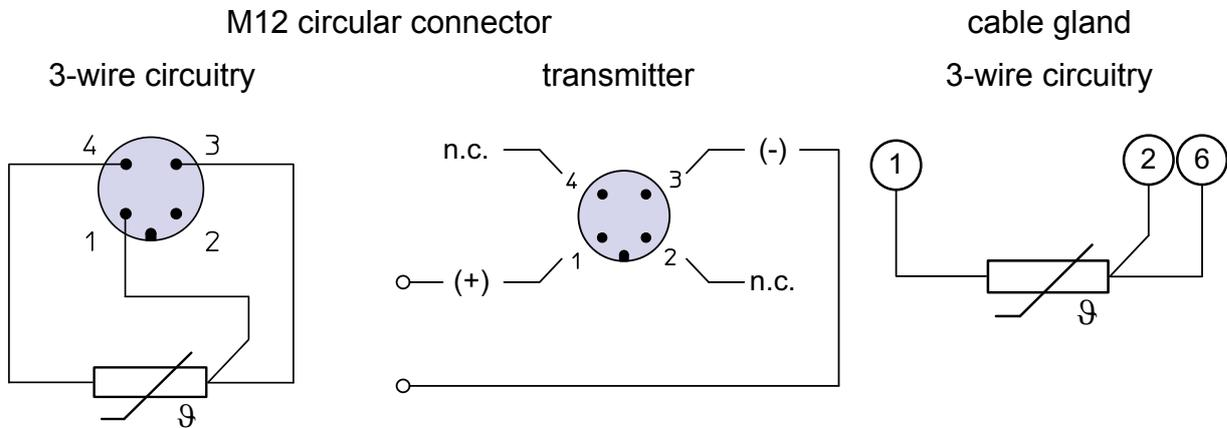
Figure 5: Variants of electrical connection
