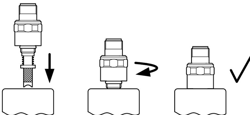
Figure 4: Mounting steps for the measuring insert
