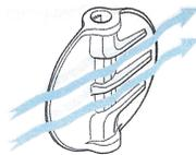
**Self-aligning stem seal through backup ring**
