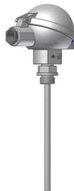
Thermocouple with integrated head transmitter 4-20mA. Designed to measure temperatures in industrial environments with gaseous or liquid media, eg. Air, steam, gas, water or oil in a stream. Temperature: -200 ° C to 600 ° C. Max 60bar and media speeds of up to 25m / sec (air) or 3m / sec (water). Welded bottom 9mm 316SS acid resistant protection tube. Welded process connection 1/2 "BSP. Aluminium connection head DIN B. gland M20x1.5mm included. Insertion length as required.
