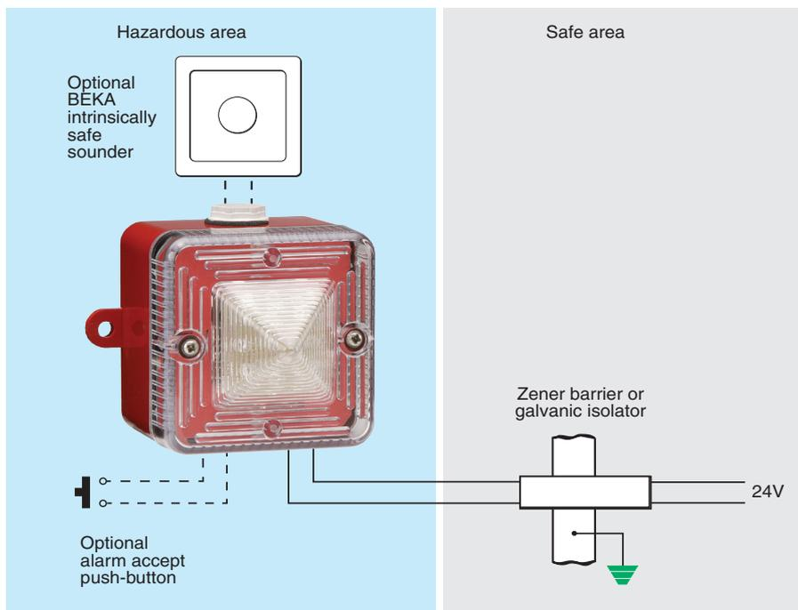
The BA386 is an intrinsically safe field mounting beacon which produces a bright flashing warning signal in a hazardous area. This beacon is significantly less expensive than the traditional Xenon devices, although it has a similar light output, flashes more frequently and is available in five different colours.
