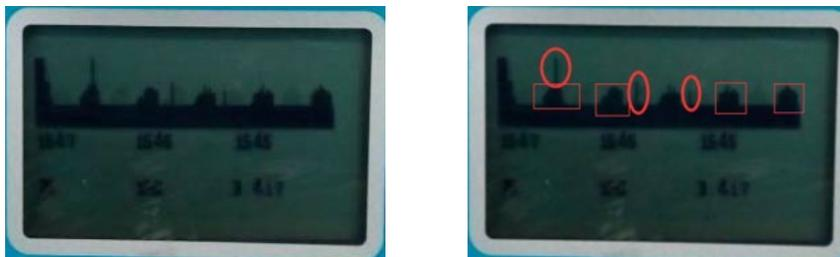
Fig. 9 Echo Pattern under Interference of Frequency Converter
