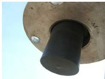
**06. Place a spacer of the same inner diameter under the flange**
