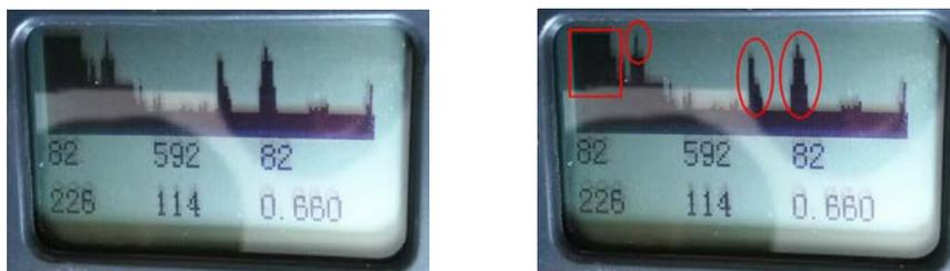
Fig. 3 Echo Pattern after Liquid Enters Blind Area
