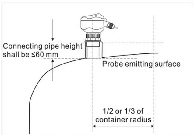
Installation on nipple joint – arch tank top
