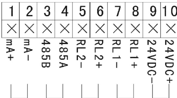
Current Output      485 Output      Relay 2    Relay 1    Connect 24V DC
