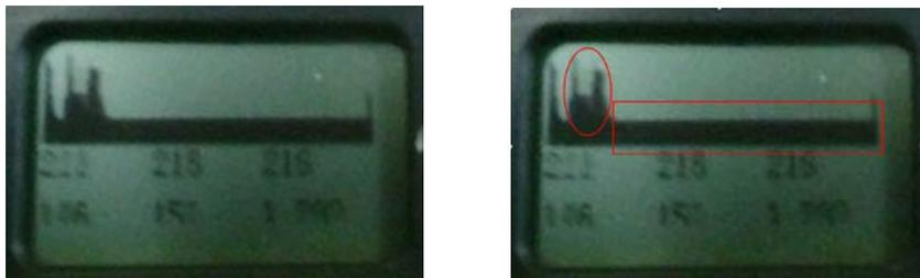
Fig. 12 Echo when Probe is Out of Connecting Pipe
