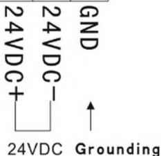
Wiring Diagram of Two-wire System
