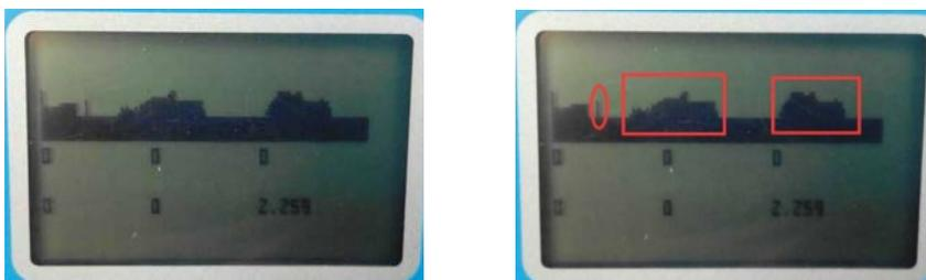
Fig. 8 Echo Pattern under Interference of Frequency Converter
