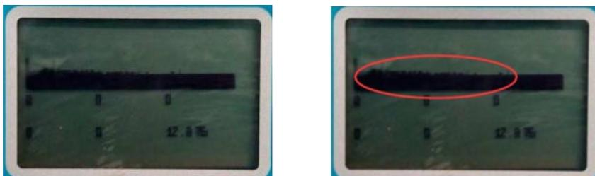
Fig. 6 Echo Pattern under Electromagnetic Interference
