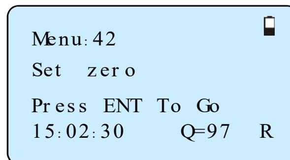
mounting location and parameters can be eliminated. The measuring accuracy at low flow is enhanced by doing this function and flow offset is eliminated.
