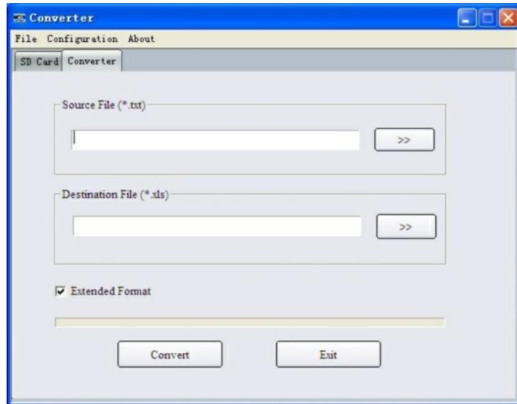
Select the file to be converted in "Source File (\*.txt)", enter the directory path and the file name in "Destination File (\*.xls)", then press "Convert". If "OK!" is displayed, the conversion is completed.
