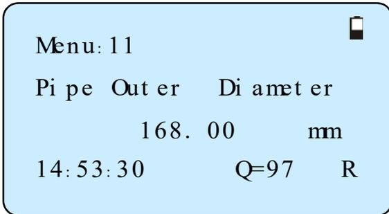
symbol “>” and a flashing cursor is displayed on the left side of the third line on the screen. The new value can now be entered. Or input the value first then press
