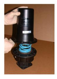
Remove spring pack by holding operating diaphragm to the lower cylinder & turn spring pack anti clockwise (This will detach the spring pack from the spindle)
