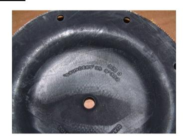
To refit diaphragm to spindle angle diaphragm, turn and push to locate
