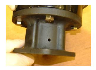
Refit cover. Slot cover to align with front port.
