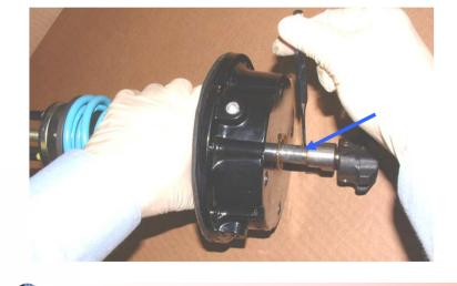
Hold master spindle secure using pin punch located in the master spindle. Turn spring pack in a anti-clockwise direction to remove.
