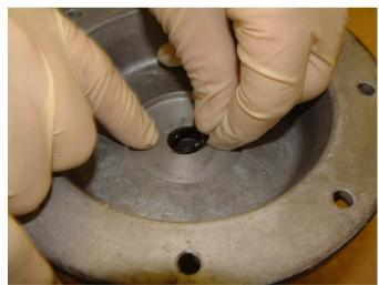
Remove securing screws from bonnets
