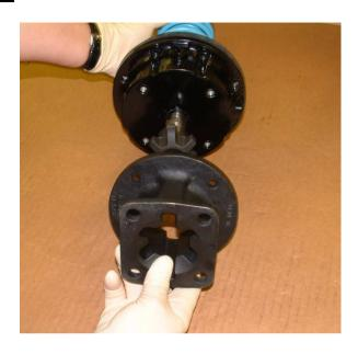
Refit bonnet to lower cylinder using securing screws.
