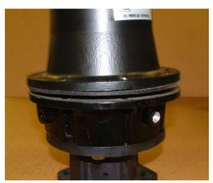
To re-fit bring the reinforcing plate to the underside of the cover by rotating the spindle clockwise. This procedure will lower the cover to aid assembly.
