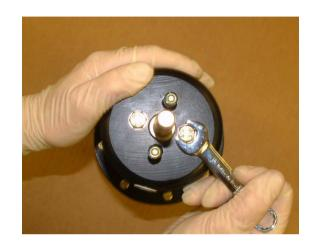
Remove cylinder/cover nuts, bolts & washers
