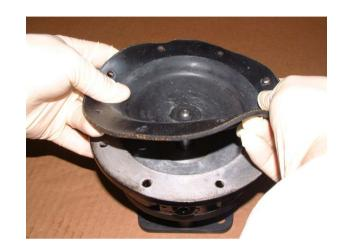
Lift to remove clamp washer from spindle
