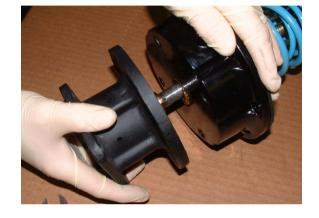
Remove bonnet from spindle compressor assembly
