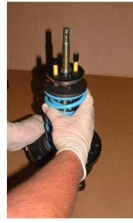
Hold spindle assembly with spanner.
