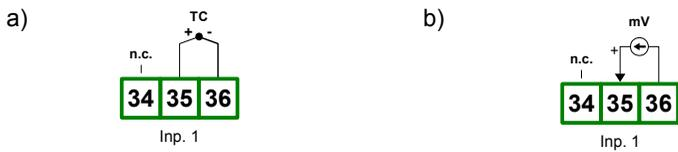
Fig. 4.15. External connection for channel no 1:
