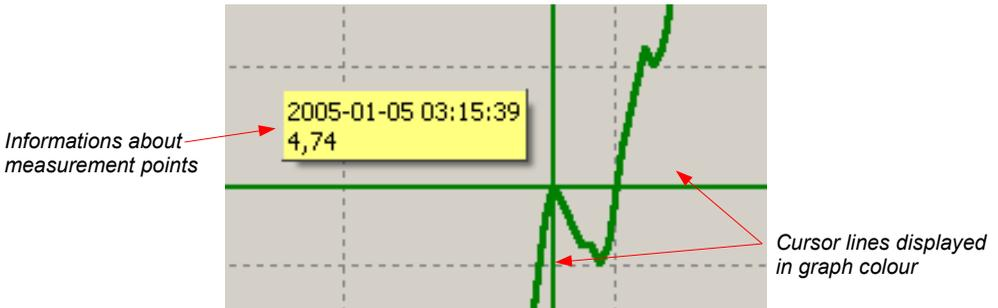
Fig. 3.9. Graph with special tracking cursor
