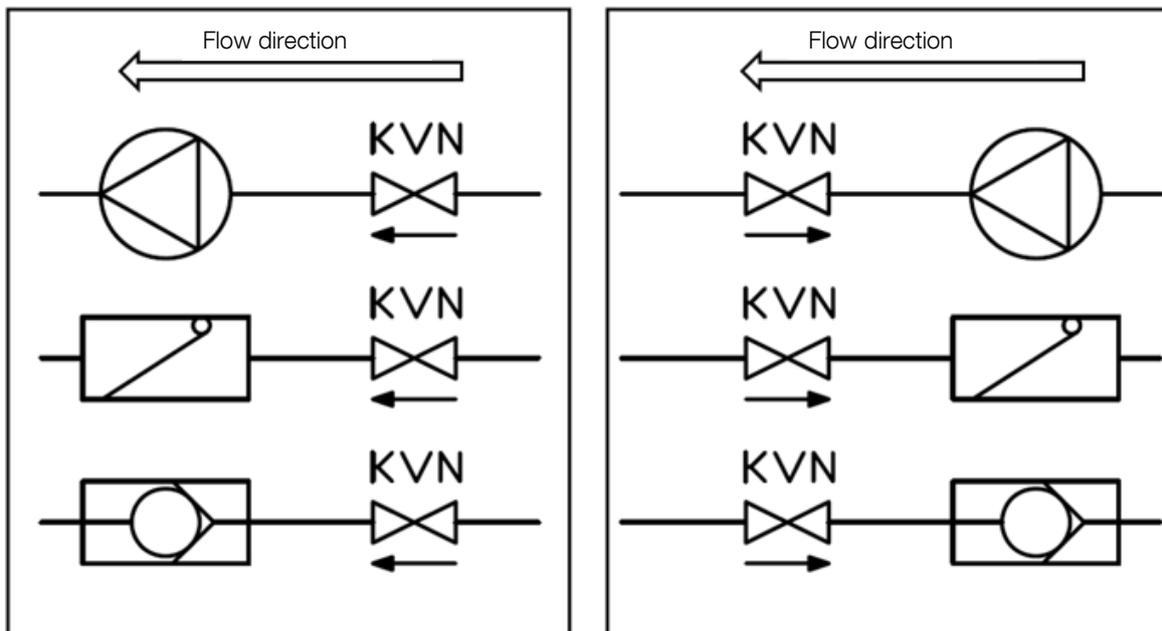
Direction of installation in front of the components
