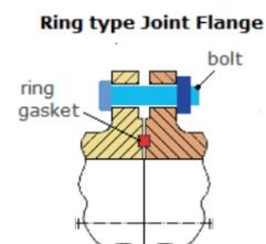
RTJ flanges have grooves cut into their faces which accept steel Ring Gaskets.
