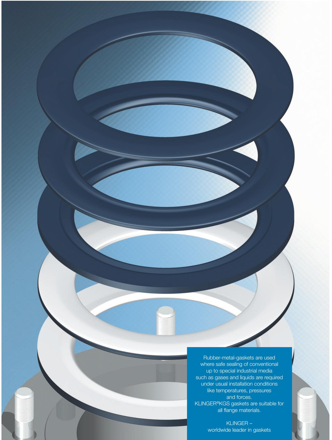
Rubber-metal-gaskets are used where safe sealing of conventional up to special industrial media such as gases and liquids are required under usual installation conditions like temperatures, pressures and forces. KLINGER®KGS gaskets are suitable for all flange materials.
