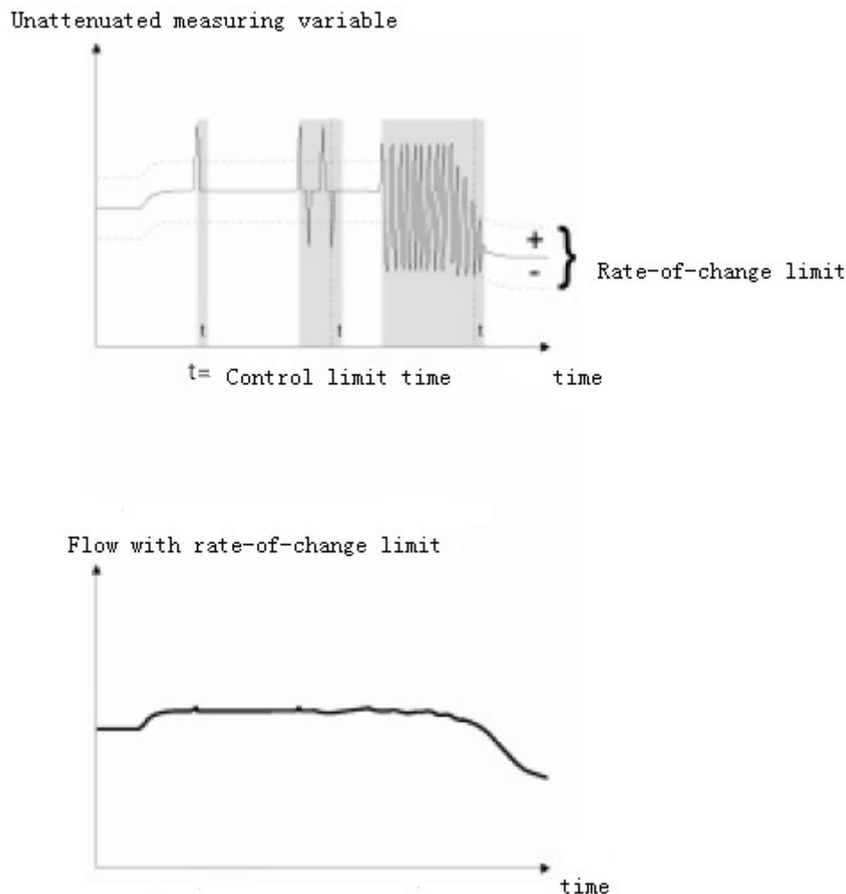
Fig.6.2 Example for the effect of rate-of-change limit
