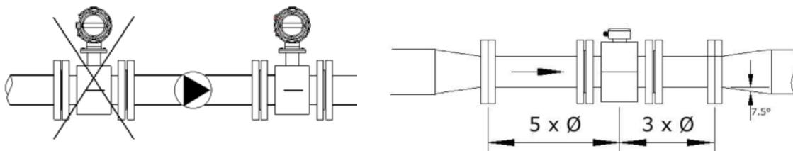
**Avoid Installing Upstream of a Pump**
