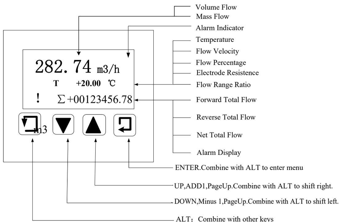
Fig. 6.1 Keypad and LCD for Display version
