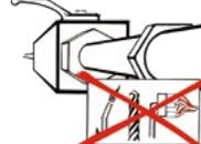
**No welding, drilling etc.**
