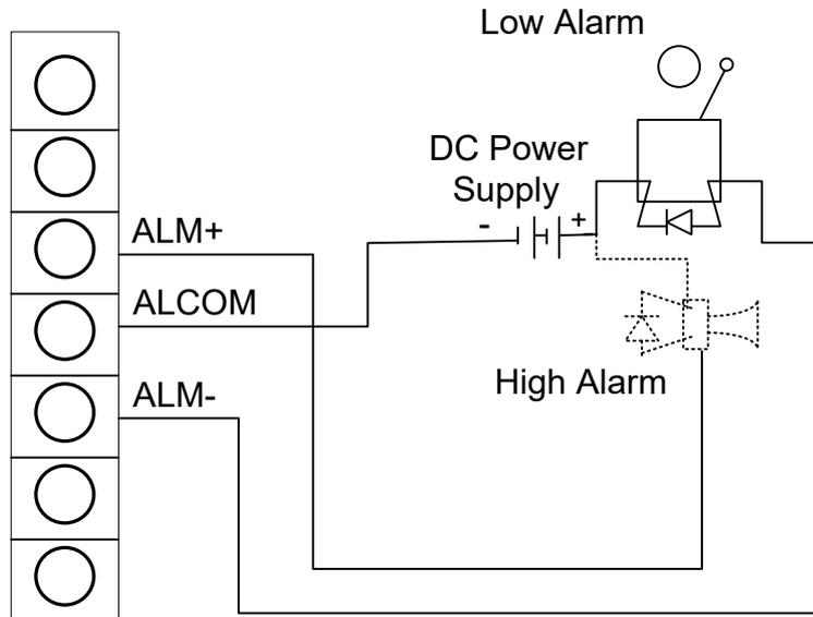
Fig 2.5 (c) Example of alarm output
