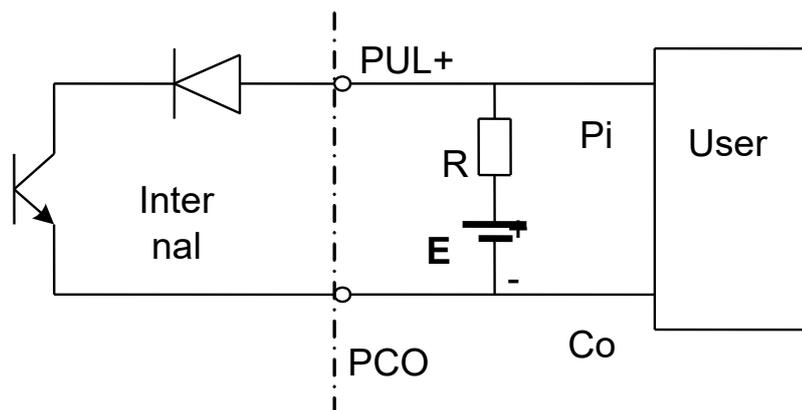
Fig 2.7 Digital Output Direct
