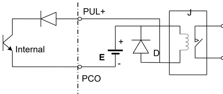
Fig 2.9 Connection with relay (e.g.
