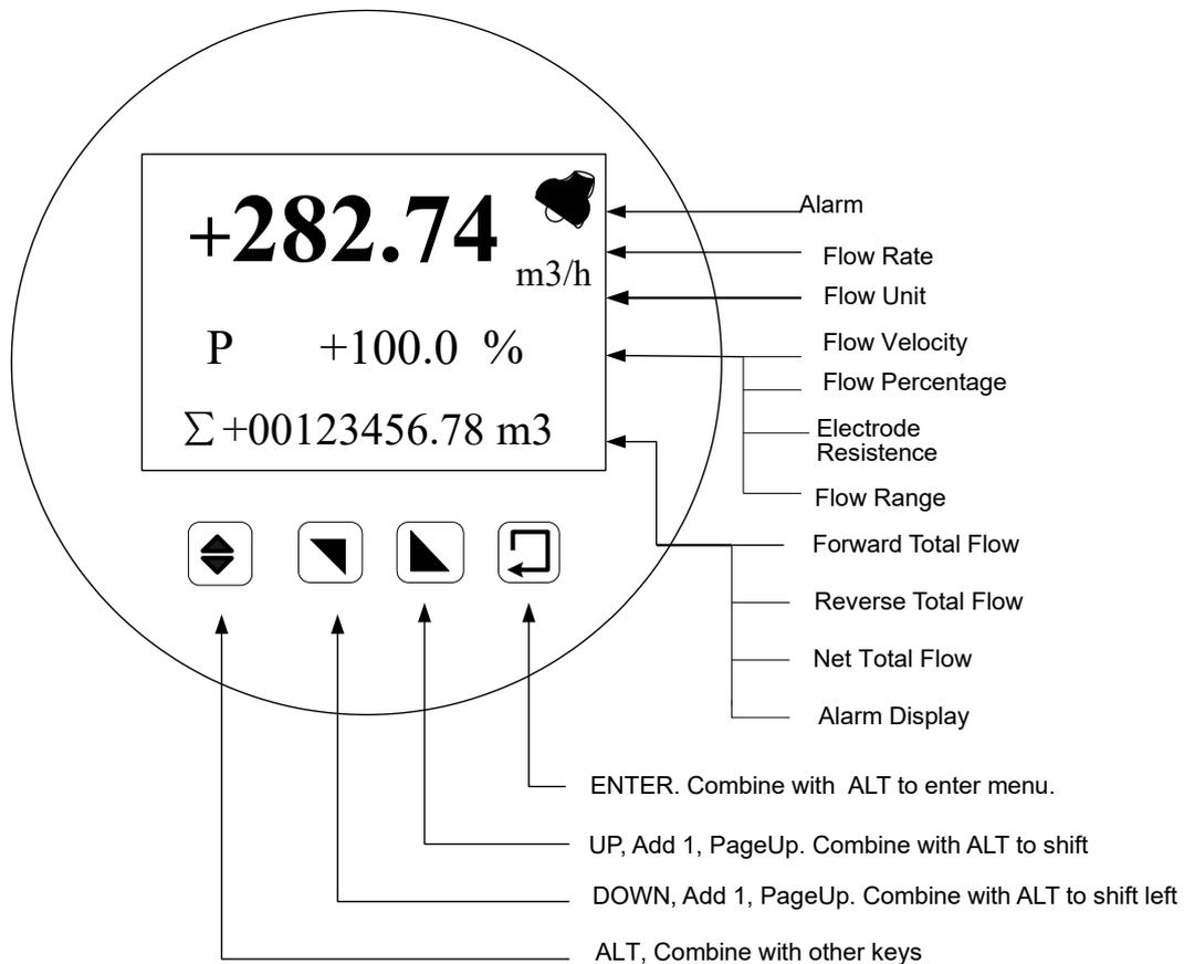
Fig 2.1(b) Compact Type: Keypad and LCD
