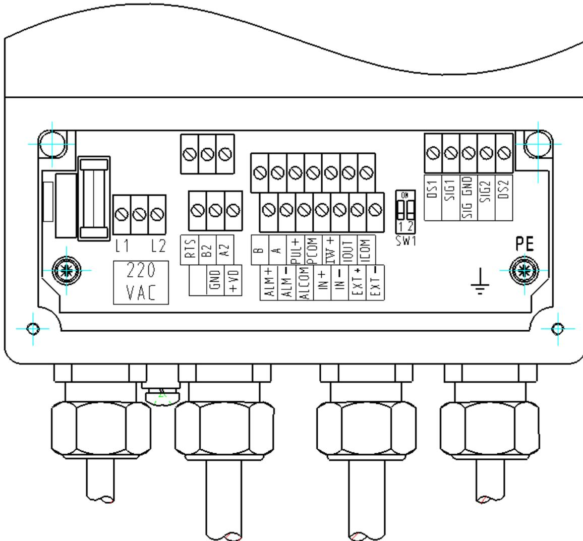
Fig 2.2(a) Remote Type: Terminals and Marks
