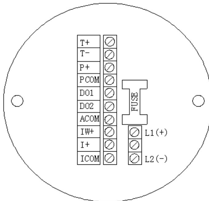
Fig 2.2(b) Compact Type: Terminals and Marks
